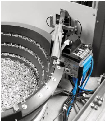
Figure 4.1: Vibration feeder for storing and sorting screws
