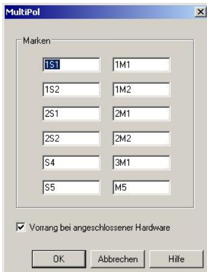
Figure 6.19: Dialog box of the multi-pin plug distributor with the labels changed
